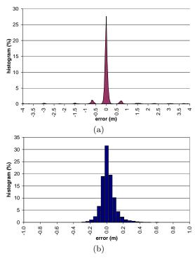
Figure 5: Error distribution of q-ranges (12000 m<sup>2</sup> experiment) obtained using (a) regular and (b) iteratively corrected ranging.
