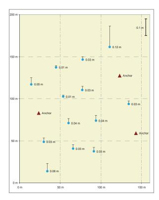
Figure 6: The setup for the 12000 m<sup>2</sup> experiment showing the anchors (large triangles), motes (small circles) and errors bars.
