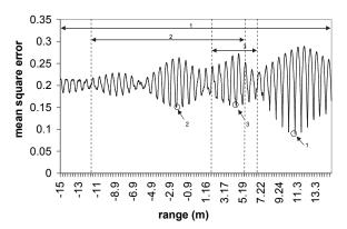
Figure 4: Phase-offset discrepancy function in a severe multipath environment. The numbers show the search intervals of consecutive error correction iterations and the corresponding minima. The spot labeled 3 is the real solution.
