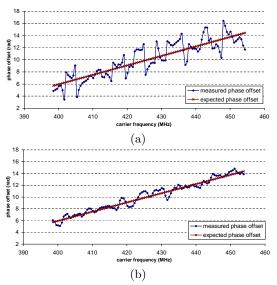
Figure 2: Phase offset measurements on 120 channels with vertical monopole antennas directly on the ground (a) and 1.3 m elevated (b).
