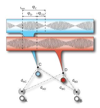
Figure 1: Radio-interferometric ranging technique.
