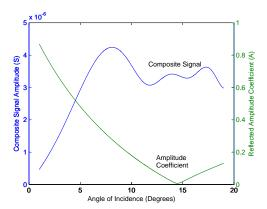
Figure 3: The reflection coefficient and the amplitude of the composite signal for vertically polarized waves. The composite signal is shaped by the interplay of the decreasing ground-reflection coefficient, and the phase offset and attenuation change due to the increasing distance the reflected signal travels.
